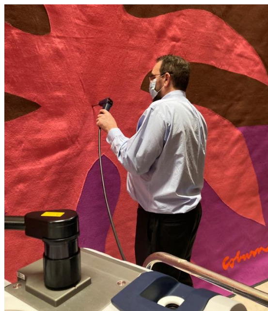
Figure 3: Dr Brad Swarbrick collecting NIR spectroscopic data from the Curtain of the Sun.
