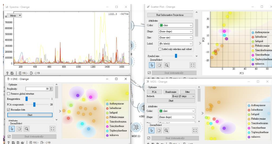
Figure 7: Result of PCA, tSNE, MDS analysis of blue pigment Raman spectra by Orange Data Mining Software
