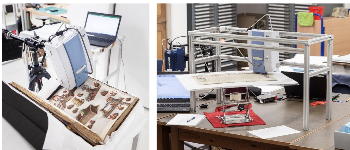
Figure 1: ER-FTIR analysis of manuscripts by using either a tripod or a tetrapod
