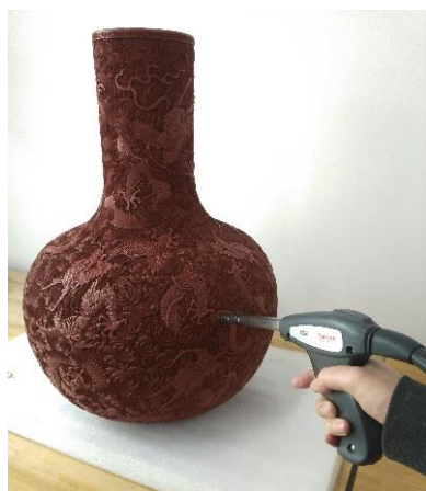
Figure 1: Collecting the NIR spectra noninvasively from a carved lacquerware of Qing Dynasty by a fiber-optics
